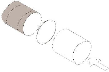
Inlet connection with the same  $\varnothing$  dimensions as the inlet bag.
