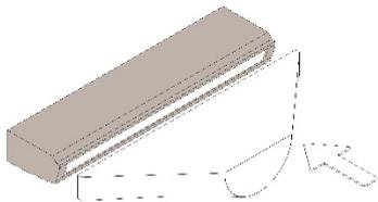
Inlet connection directly via ventilation system.
